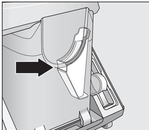
A removable filter frame is located in the dust container. This should be cleaned if it is obviously dirty.
